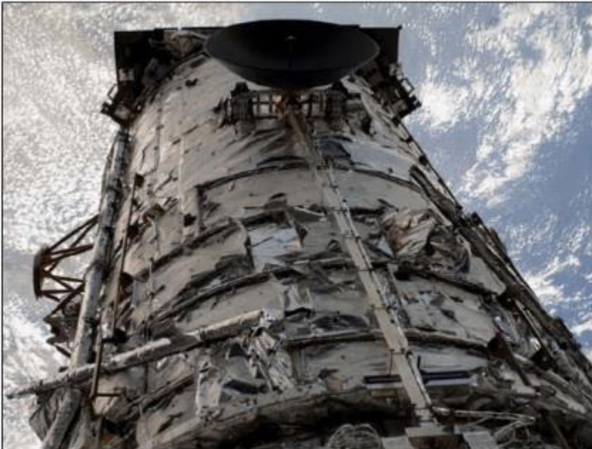
Severe degradation to the aluminized-Teflon outer layer of multilayer insulation on the Hubble Space Telescope after 19 years of space exposure.
