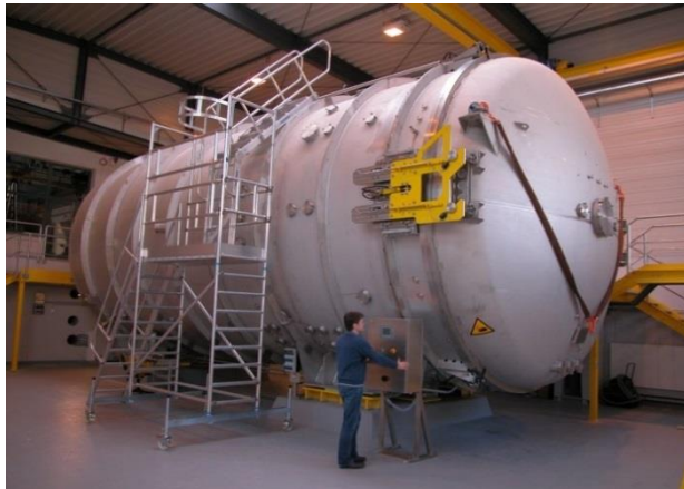
Vacuum chamber of the STG-ET facility (DLR – AS RFZ Göttingen, Germany)
