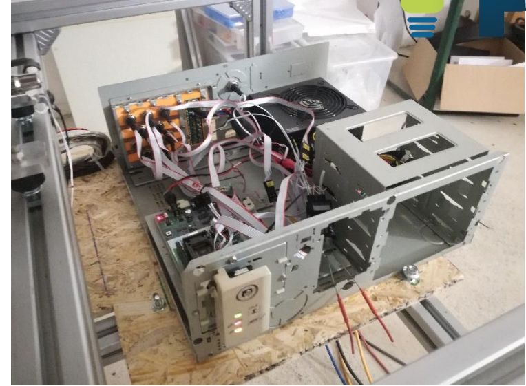
Central processing unit and switching board
