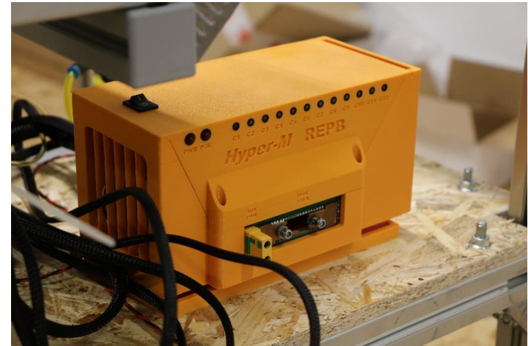
REPB central electric power bank
