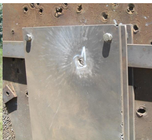
HEDP ATIR Ammunition tests armored vehicle steel plate – penetration through three armored steel plates
